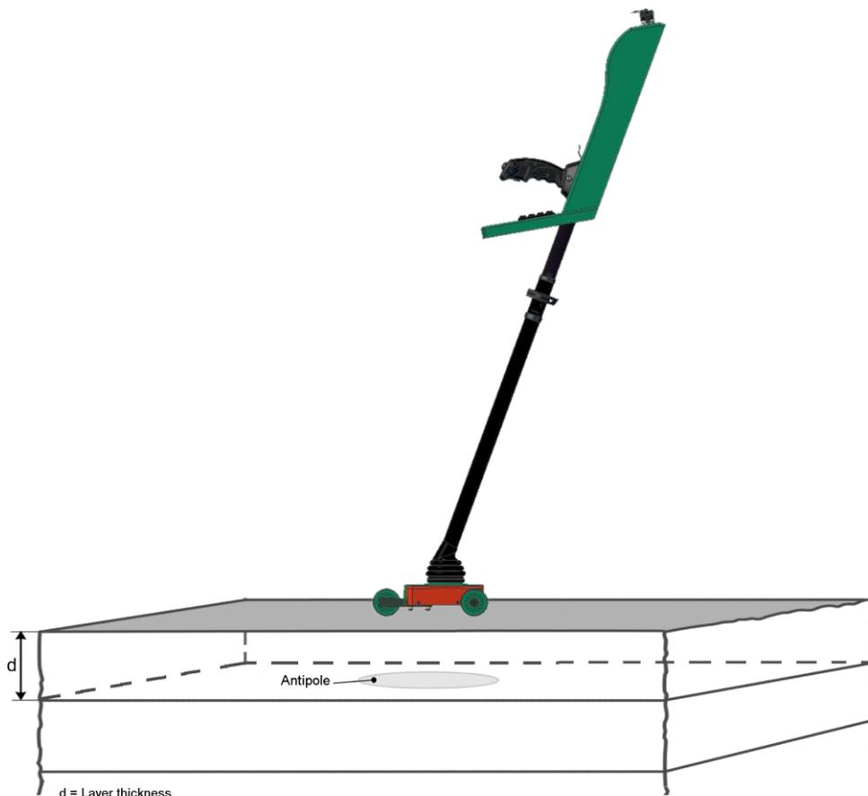
**Figure 4: Electromagnetic thickness measurement using pulse induction technology**
